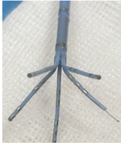
Figure 1. Ex-vivo catheter image showing four normal splines and one ruptured spline.
